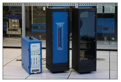
Due to the limited capability to mount GTIO cards within the Portable cubicle (there is room for one GTFPI card), a separate I/O cubicle can be provided to house additional GTIO cards. The portable I/O cubicle has a 24 V power supply to run the GTIO cards and casters so that it can easily be moved from place to place. A flight case is also available for the portable I/O cubicle as an optional item.
